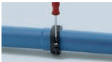
Now tighten the screw. The maximum admissible torque is 7 Nm. Fittings in the dimensions DN/OD 32–90 must be pulled apart by 5 mm before the POLO-KAL NG ASV is installed. (FIGURE 3)
